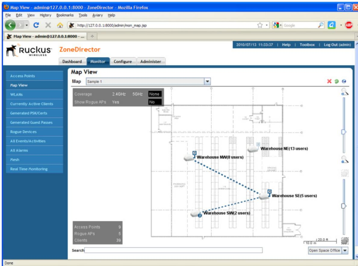
Figure 2: The ZoneDirector 1200 provides a detail map view that lets administrators quickly see the Wi-Fi network topology for all Ruckus Smart Wi-Fi access points.
